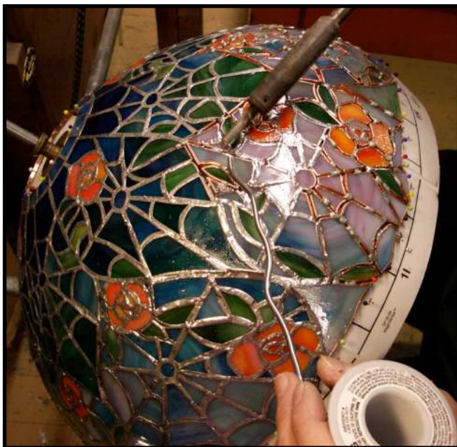
Glass pieces tack soldered and flat seamed
