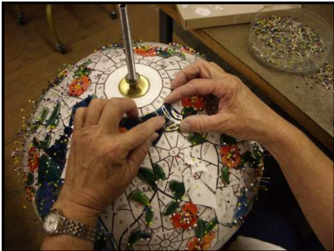
MagicStrips™ attached to form Pattern cut out and pinned on form to check for fit Glass cut and held in place with glass headed pins
