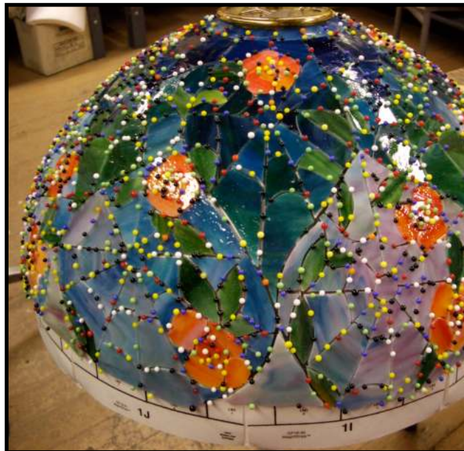
Glass pieces pinned in place, ready to foil and solder
